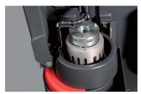
The powerful German Schabmueller maintenance free AC Drive motor in combination with the German Kordel gearbox, Intorqe brake and Wicke drive wheel give best performance, efficiency and reliability to reduce the running costs!
